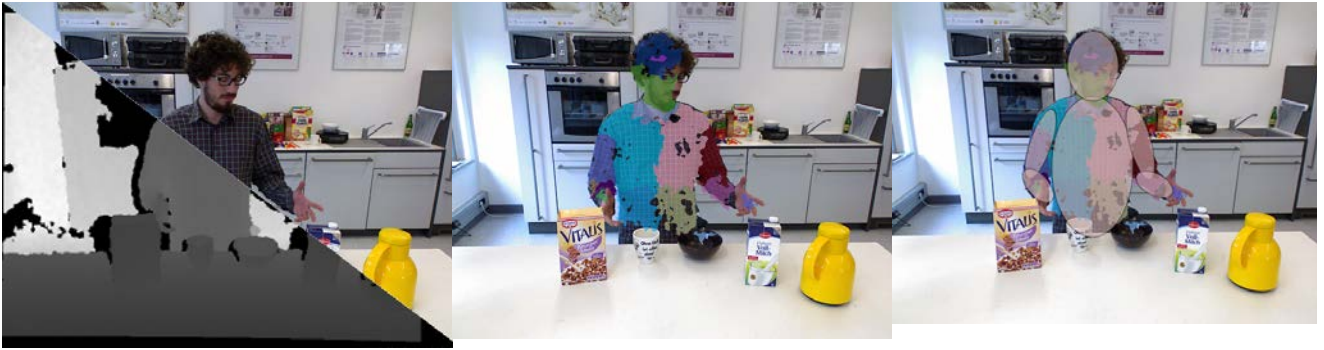
Figure 11: Human tracking pipeline from raw RGB-D input (a), over segmented and labeled regions of the human body in the point clouds (b), to an ellipsoid-based representation in the plan-based controller(c).
