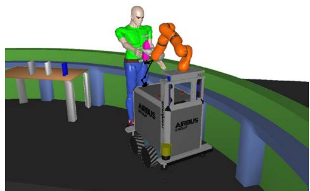
(b) A placement configuration computed by a "hand-over placement planner"
