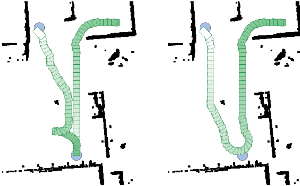
Figure 2: Mobile robot moving to two subsequent goals: (a) separate planning towards each goal, (b) combined planning for the action sequence composed of two goal regions. As expected, the combined planning is superior to the separate planning as it can avoid the unnecessary turning manoeuvre.
