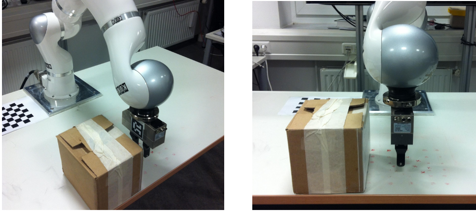
Figure 2: 7 DoFs KUKA/DLR Lightweight Robot (LWR) in its initial pose for an object pushing task: The aim of this RL task is to push a box to a given goal position along the edge of a table. Physical contact between robot end-effector and object will be established soon after the movement is initiated.
