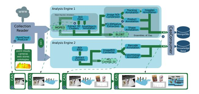
Figure 3: Example of a pipeline execution in RoboSherlock showing how the content of the CAS changes over time and the main parts of the system: CAS producer, Analysis Engines, Cas Consumers and Annotators. Note: the locations of MOPED [4] and Blort [5] are marked with different color because at the moment they represent a possible integration
