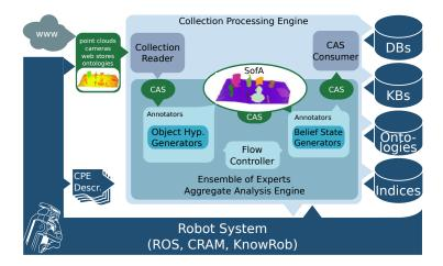
Figure 2: Schematic overview of our UIMA-based object processing framework.
