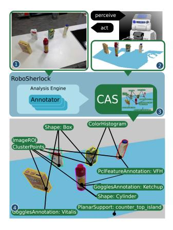
Figure 1: Perception as Unstructured Information Management: Common Analysis Structure (CAS) holds the original high-res camera (1) and depth (2) images, which act as input documents for our RoboSherlock system (3). The CAS (4) also contains information concerning known structure (such as the 3D semantic map, light blue), and filtered regions (gray), as well as Annotations referencing various parts of the document (green labels).
