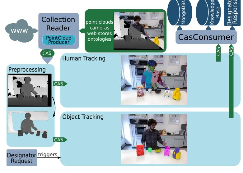
Figure 1: Overview of the pipeline of AEs used within the context of SAPHARI. The collection reader at the very beginning, the preprocessing AE and subsequent the tracking AEs, running in parallel. They forward informations to the CASConsumer which (a) stores informations in a mongo database, (b) in a knowledgebase, or/and (c) returns information as a reponse to a request. Perceived bodyparts and objects are marked by a colored overlay.
