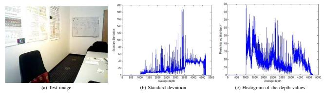
Fig. 1: Variation of depth values around per pixel means averaged over all pixels of the same depth
