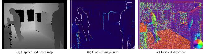
Fig. 4: Depth map with large gaps (taken from the video sequence shown in Fig. 3) and gradient of the inpainted depth map
