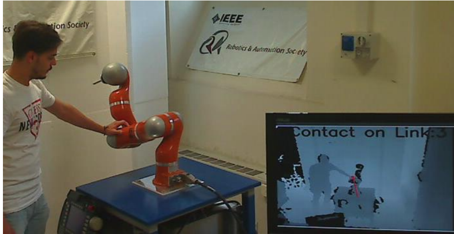
Figure 25 Balanced force on link 3 along the z-axis between human and robot during a collaboration with stiffer parameters. Depth image, with the vector of estimated contact force highlighted in red (bottom right).
