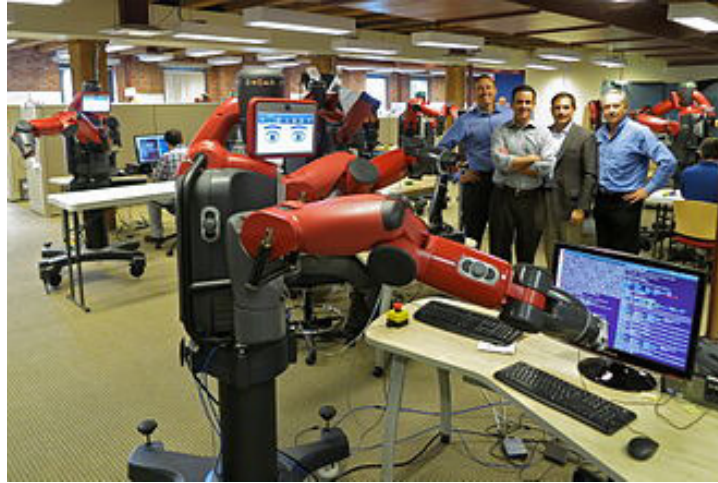
Figure 1: Baxter: the adaptive, collaborative manufacturing robot realised by Re-thinkRobotics
