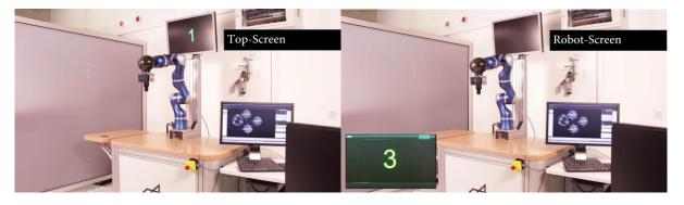
Fig. 7: Displaying information about the Task State on the Top-screen (left) or the Robot-screen (right)
